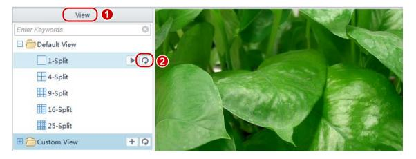
After sequence display is enabled for a default x-split view, the live videos of cameras in the camera list are played by turns in x windows.
