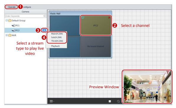
Alternatively you can drag a camera to the channel to display its live video.
