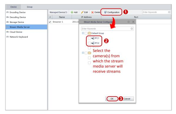
The stream media server will receive streams from the specified cameras and display the stream receiving records.
