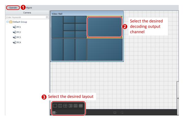
You can drag multiple cameras to a decoding output channel for which the screen is split. This implements the display of multiple live videos in a single decoding output channel.
