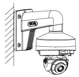
Figure 2-10 Fix the Camera to Wall Mounting Bracket
