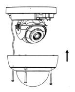
Figure 2-7 Install Bubble
