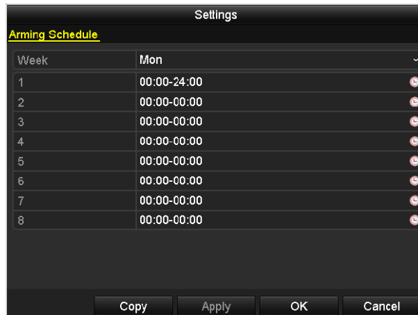
Figure 7-17 Set Arming Schedule of Alarm Output
